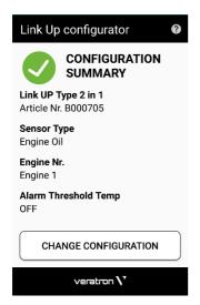
2. After the readout, the App will show the "Configuration Summary", which displays all the current settings of the device.
